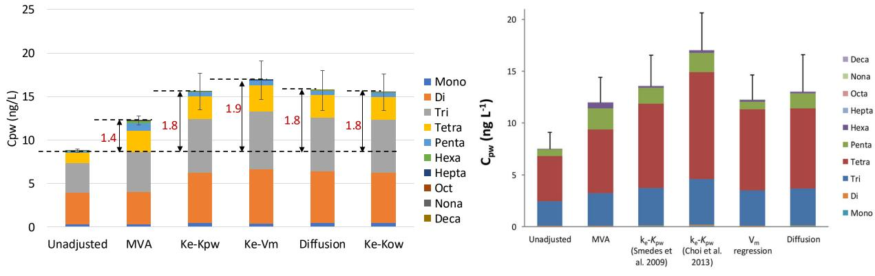
$C_{\text{free}}$  of PCBs in upper 15 cm of unamended Lower Lower Beverdam Creek Study area sediment
